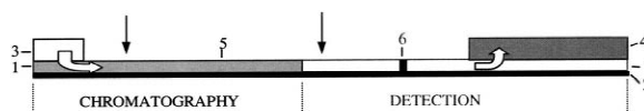
Fig. 1. Device for thin-bed chromatography. The device is composed of a membrane with separation, transport and detection zones (1). The membrane has a non-porous backing (2) on the bottom side but its upper side is open for application of reagents. The driving force for the migration of liquid is capillarity, and the flow is kept up by a buffer-delivering pad (3) and an absorbent sink (4). The separation zone (5) can be equipped with different functionalities for the desired type of chromatography e.g. ion-exchange, affinity or hydrophobic chromatography. The detection of the separated molecules can be performed by immunoassay, using an immunoaffinity zone (6), which together with a labelled reactant gives a sensitive quantitative determination of the target molecules. Other commonly utilised detection methods, such as staining of the separated molecules, can also be used.
